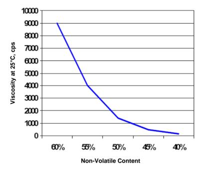
High film thickness application is related to the amount of water contained in the ready-to-use compound. Application tests did not develop cracking due to film shrinkage in the following systems:
