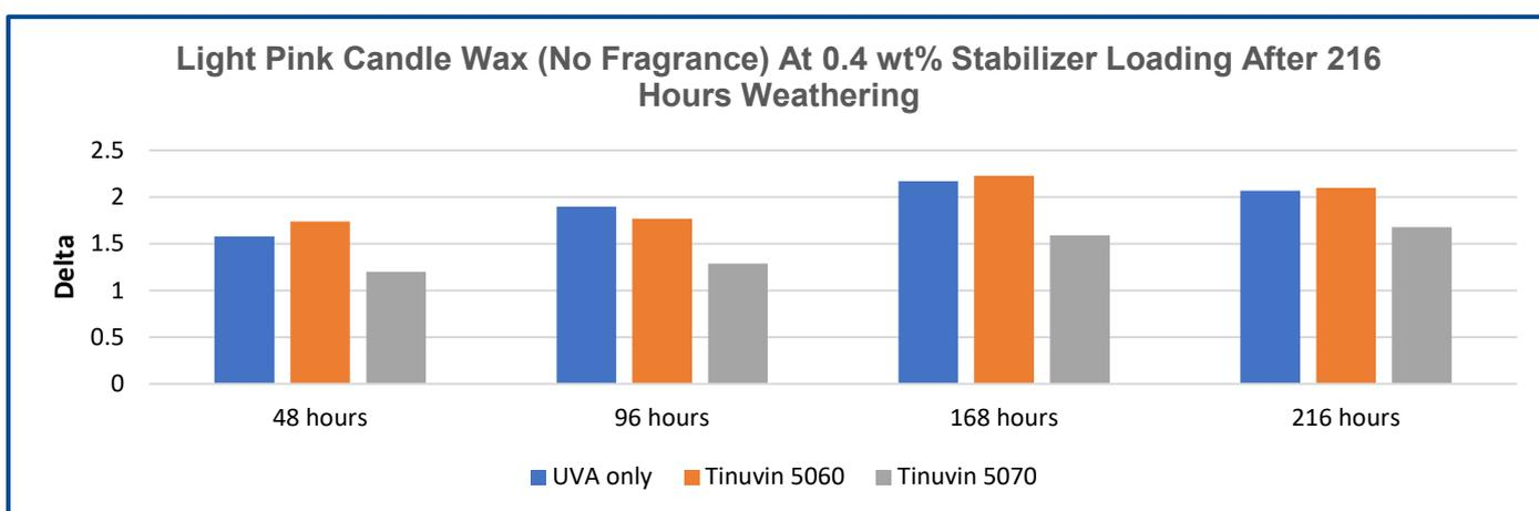
**TINUVIN 5070 has the best color stabilization and less color generation in dyed wax over time (216 hours).**
