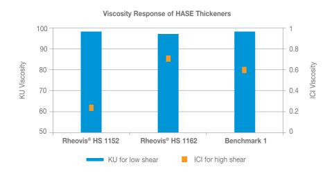
BASF's HASE rheology modifiers give the formulator the ability to tailor the coating viscosity profile to meet their specific needs. Rheovis® HS 1152 should be considered for enhancing low-shear viscosity when limited impact on high-shear viscosity is desired. In coatings where both high shear and low shear viscosity enhancements are required, Rheovis® HS 1162 is an excellent choice.
