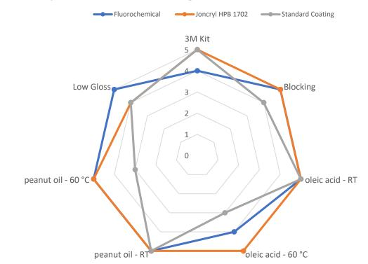
Comparison of Joncryl HPB 1702 to standard coating and FC-treated board.
