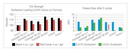
Tint strength and freeze-thaw resistance in an acrylic semi-gloss paint at 50 g/l VOC's; Hydropalat WE 3111 shows excellent tint strength development and very good freeze thaw resistance compared to APE and APE-free controls.
