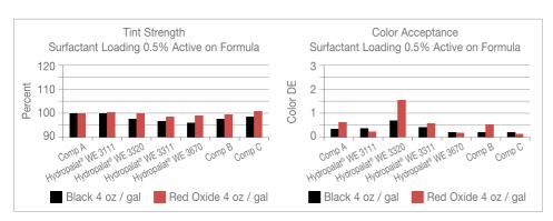
Tint strength and color acceptance in a vinyl acrylic flat paint at < 5 g/l VOC's; Hydropalat WE 3111 shows excellent tint strength development and very good color acceptance compared to APE and APE-free controls.
