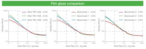
Efka® RM 1506 allows the formulator to prevent pigment settling and anti-hard caking without affecting viscosity
