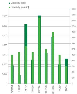
**Hardness – flexibility** / formulation: 70 parts Laromer PE 56 F, 30 parts monomer, photoinitiator: 4% blend of benzophenone and α-hydroxy ketone
