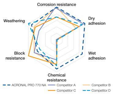
In a benchmarking study looking at more than 20 competitive water-based, 1-component direct-to-metal coatings, Acronal PRO 770 NA was a top performer for corrosion, dry adhesion, wet adhesion, and chemical resistance. It achieves a good balance of block-resistance and flexibility. Contact us for detailed test results.
